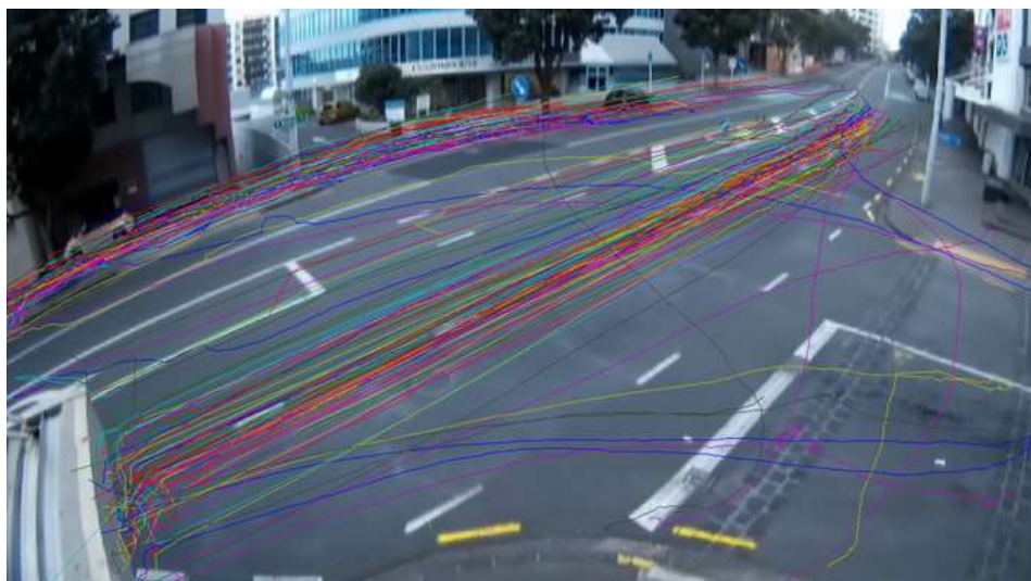
Figure 18: ANZAC Ave/ Short St - Cyclist movement through the intersection (computer vision)
