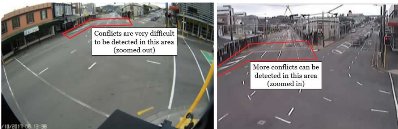
Figure 14: Camera views showing View 1 (top, with high quality, zoomed out view) and View 2 (bottom, with low quality, zoomed in view) displaying an example conflict detection zone
