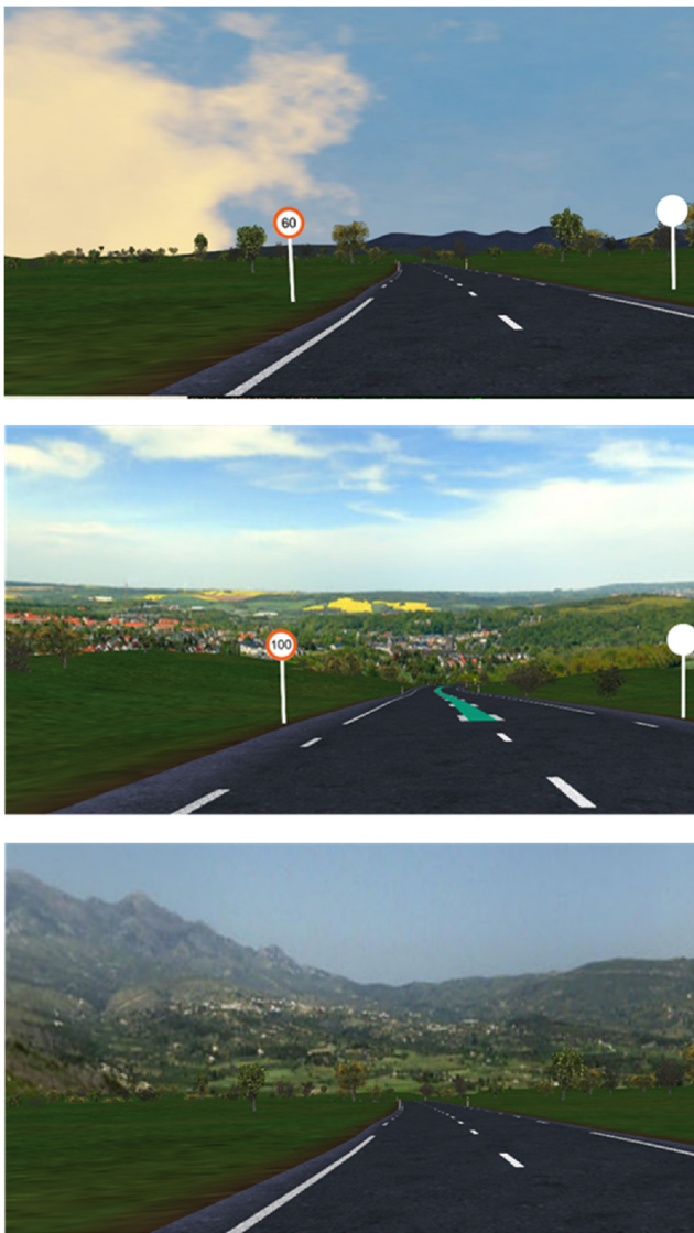
Fig. 4. The road markings and background scenery from a driver's point of view. Top: the default background (used for Session 1 trials, and trials 1, 2, & Workload Trial of Session 2) and an example of an 80–60 km/h speed transition with perceptual markings. Middle: background scenery used during Generalisation Trial, and a 60–100 km/h speed transition with perceptual markings. Bottom: background scenery during the No Signs Trial and an 80–60 km/h transition with attentional markings.
