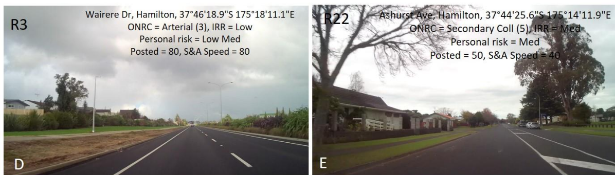
Figure 18. Two roads with poor observed speed limit credibility (typically driven at \geq 5 km/h above the posted speed limit).
